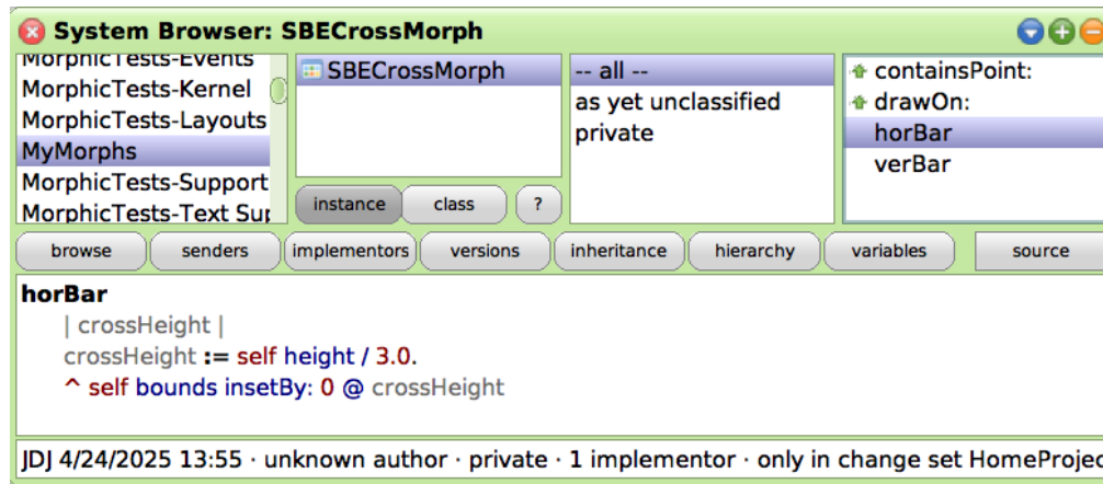
Figure 1. The Squeak Smalltalk class browser. Columns from the left: class categories, classes in the selected category, method protocols for the selected class, methods in the selected protocol. The bottom text area contains the Smalltalk source code for the selected method, which gets recompiled upon committing the edit with Ctrl-S.
